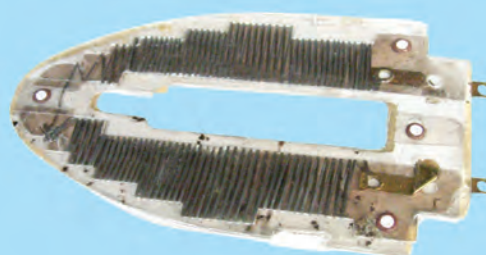
Fig. 14.11 Element of electric iron
